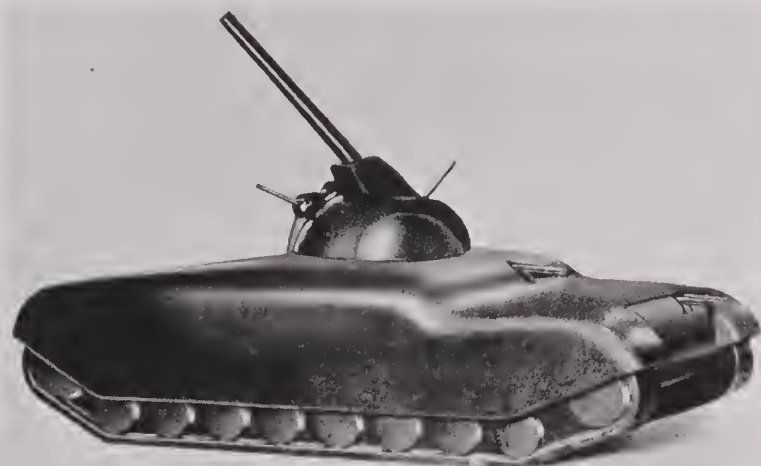
FIGURE 4. Model of IVI-D medium tank equipped with 75-mm gun.
